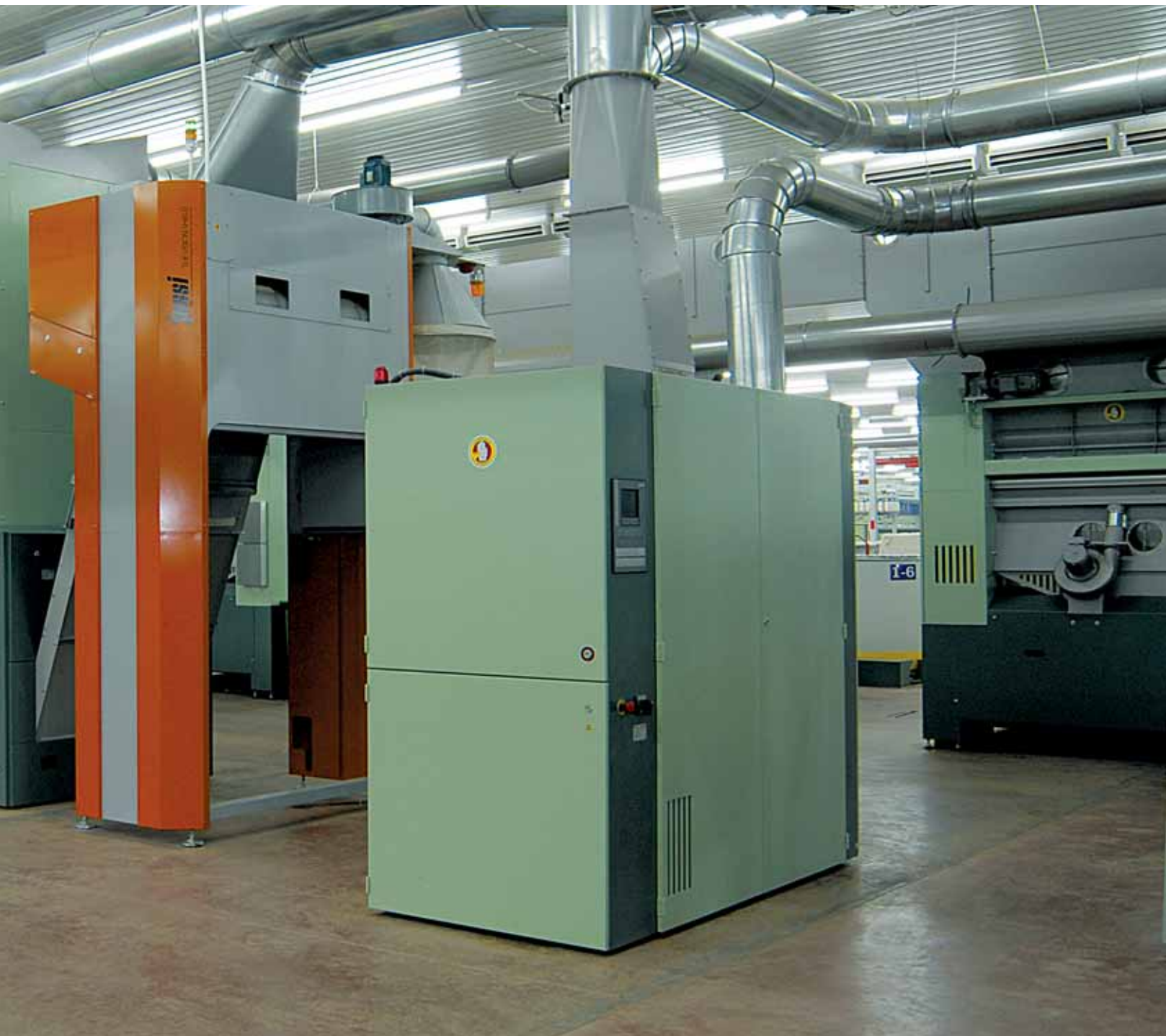
The pre-cleaner UN1clean B 12 is an integral part of the Rieter blowroom.
