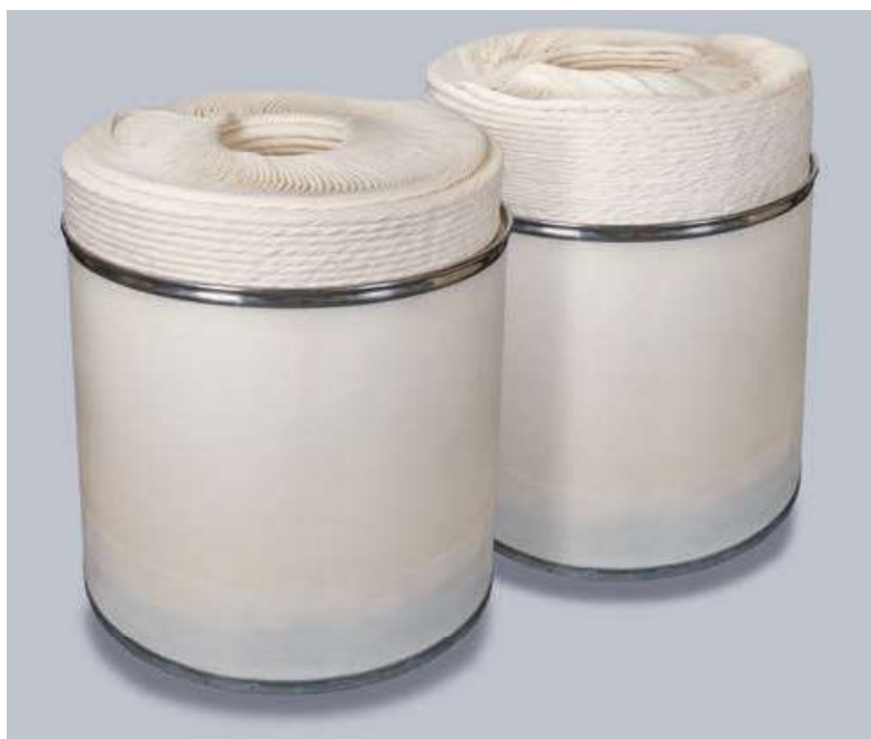
On the left, the optimized T-MOVE 2 coiling geometry and on the right, the conventional coiling geometry. Both cans contain 80 kg of card sliver.
