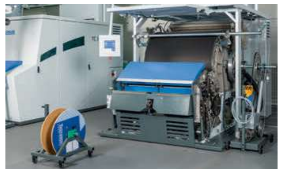
With the comprehensive Truetzschler Mounting Equipment TC-ME, all cards are optimally prepared for clothing and re-clothing.
