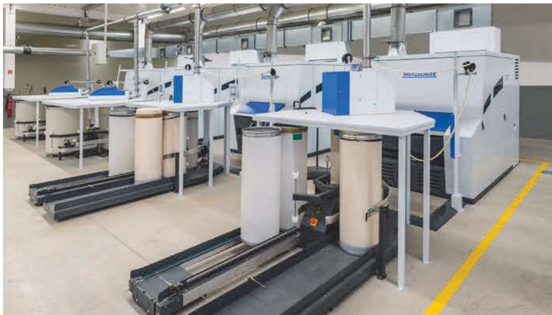
IDF 2 installation with 450 mm round cans
