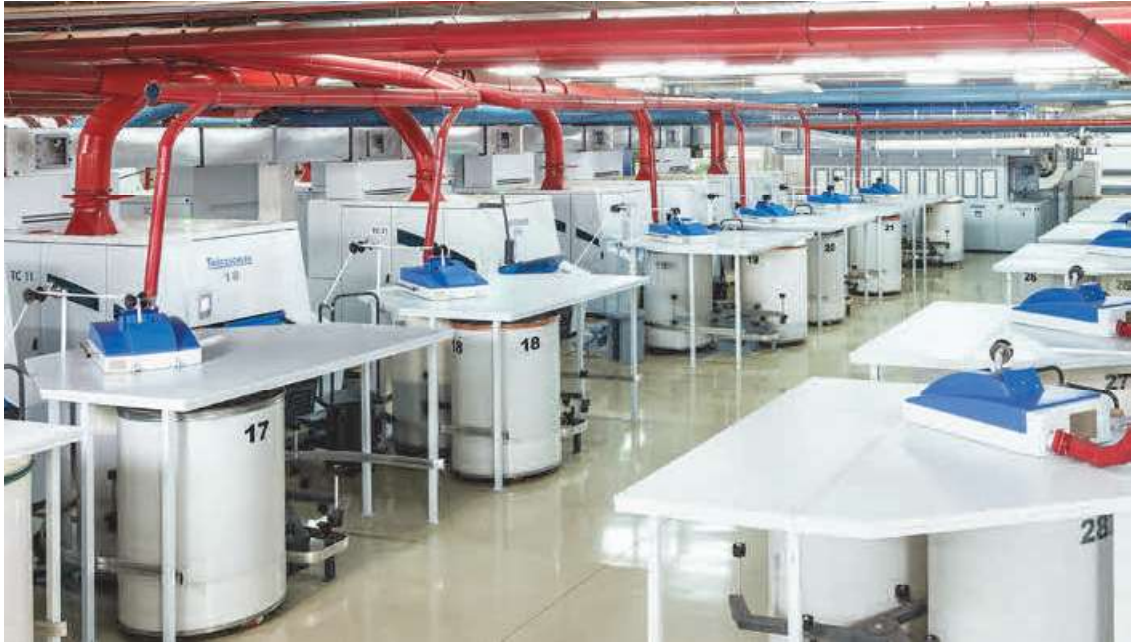
Card installation with Rotary Can Changer CCA
