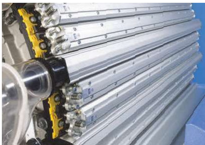
The T-CON 3 spacers can easily be replaced in just a few simple steps and thus allow a reproducible setting of the carding segments.
