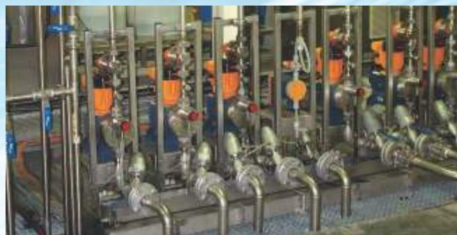
Online pH & Redox potential indicator and controller provided with the machine also ensure uniform colour shade. This guarantees process reliability and reproducibility of the results in subsequent batches.
