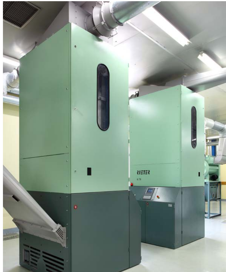
A 79 UNIstore with TVS foreign fibre detection
