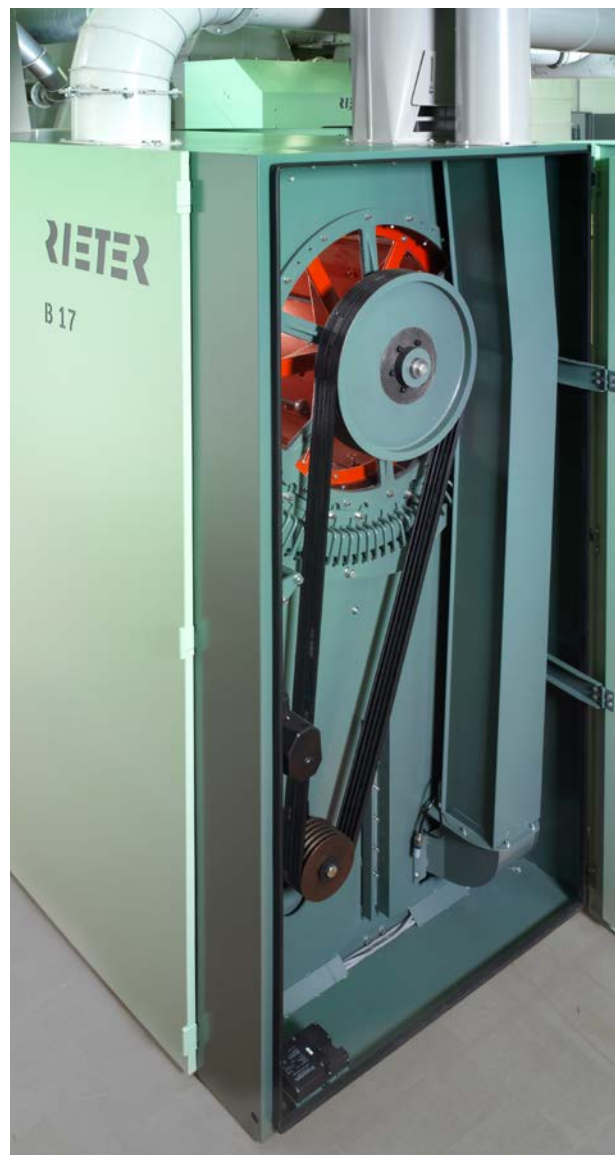
Simple setting of the grid bars at the UNIClean B 17 with VARIOset
