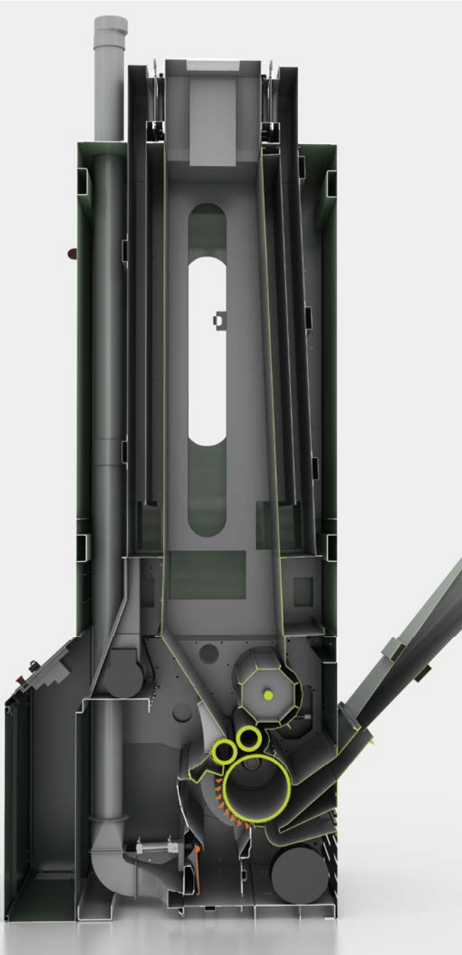
Modular construction of the A 79 UNIstore
