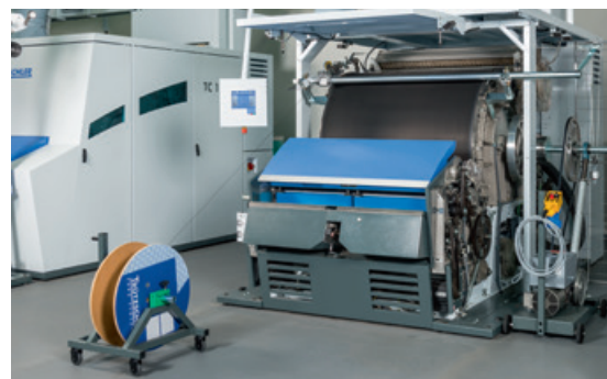
With the comprehensive Truetzschler Mounting Equipment TC-ME, all cards are optimally prepared for clothing and re-clothing.
