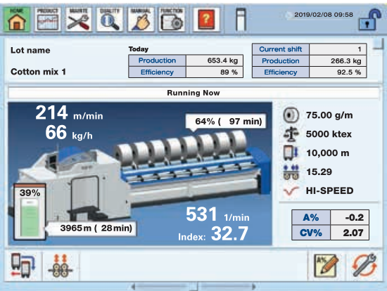
Permanent sliver control with DISC MONITOR. The data are shown online on the machine display.
