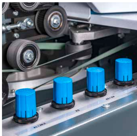
These controllers allow easy and reproducible settings of the top roller loads. A special sensor monitors the pressure.
