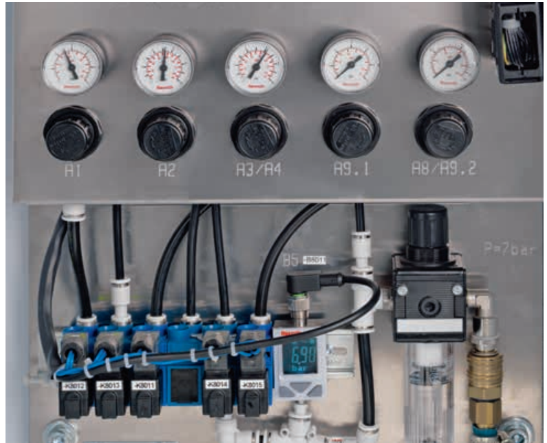
These controllers allow easy and reproducible settings of the top roll loads. A special sensor monitors the pressure.
