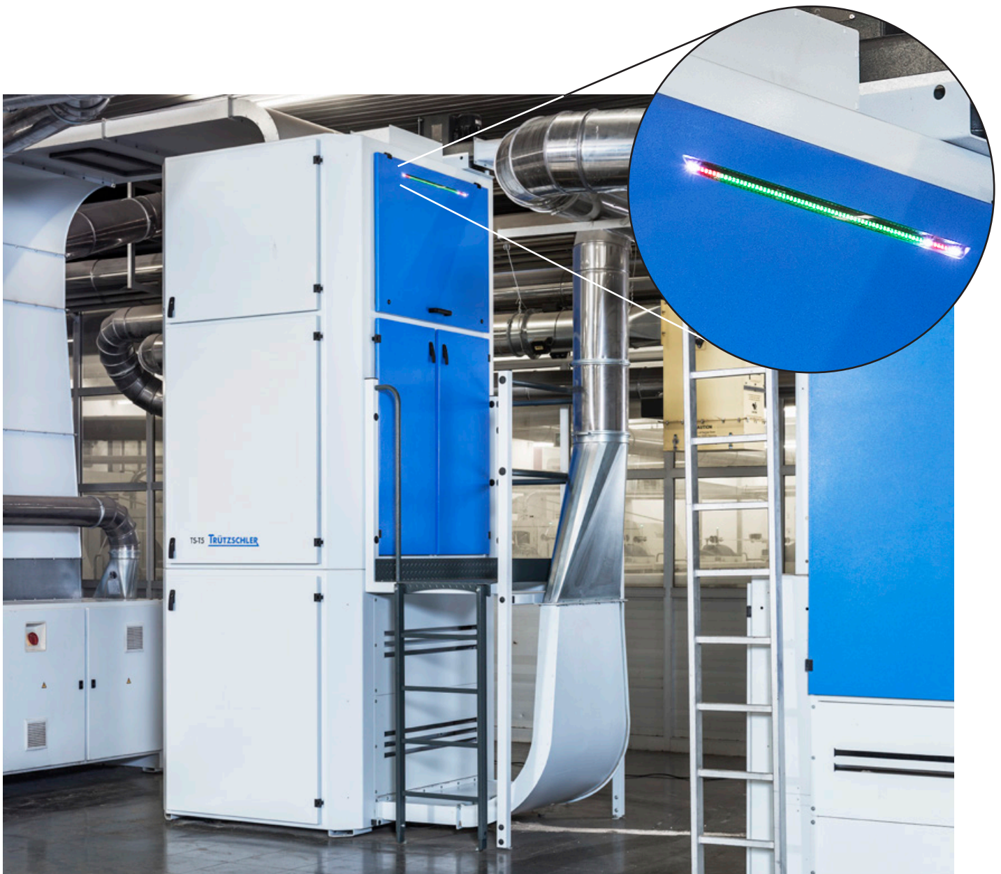
The Truetzschler remote display T-LED makes the machine conditions visible from far away.
