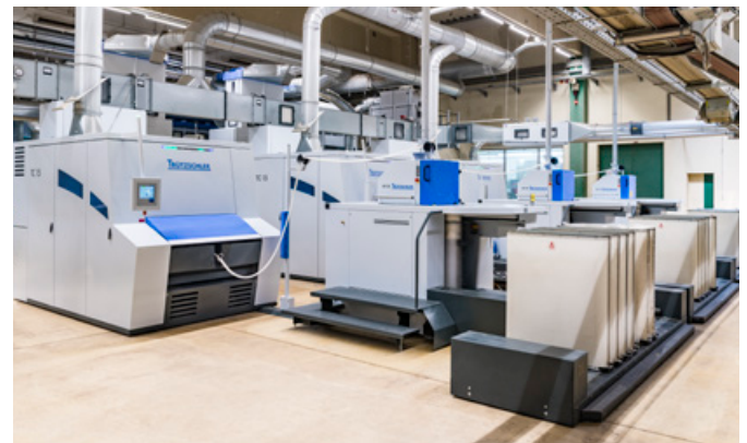
The ideal solution for rotor spinning: IDF 2 with rectangular can changer
