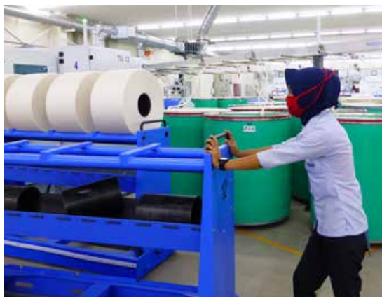
User-friendly handles facilitate the transport of the lap carriage.
