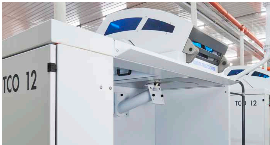
The picture shows the mounted suction nozzle for the sliver suction on the Comber TCO 12.
