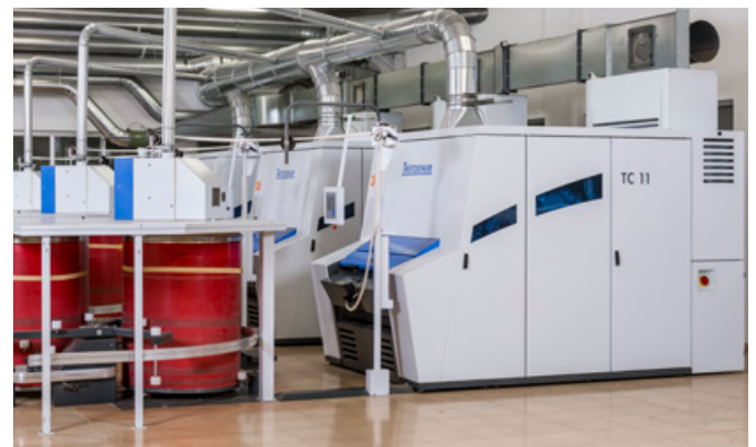
Perfect for airjet spinning with a subsequent autoleveller draw frame passage: the IDF 2 with 1,000 mm cans.
