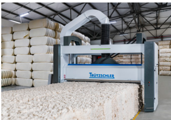
Hard-pressed waste bales that are difficult to process are worked off here. The gap-free appearance of the bale surface is perfect even at a production rate of 2,400 kg/h.
