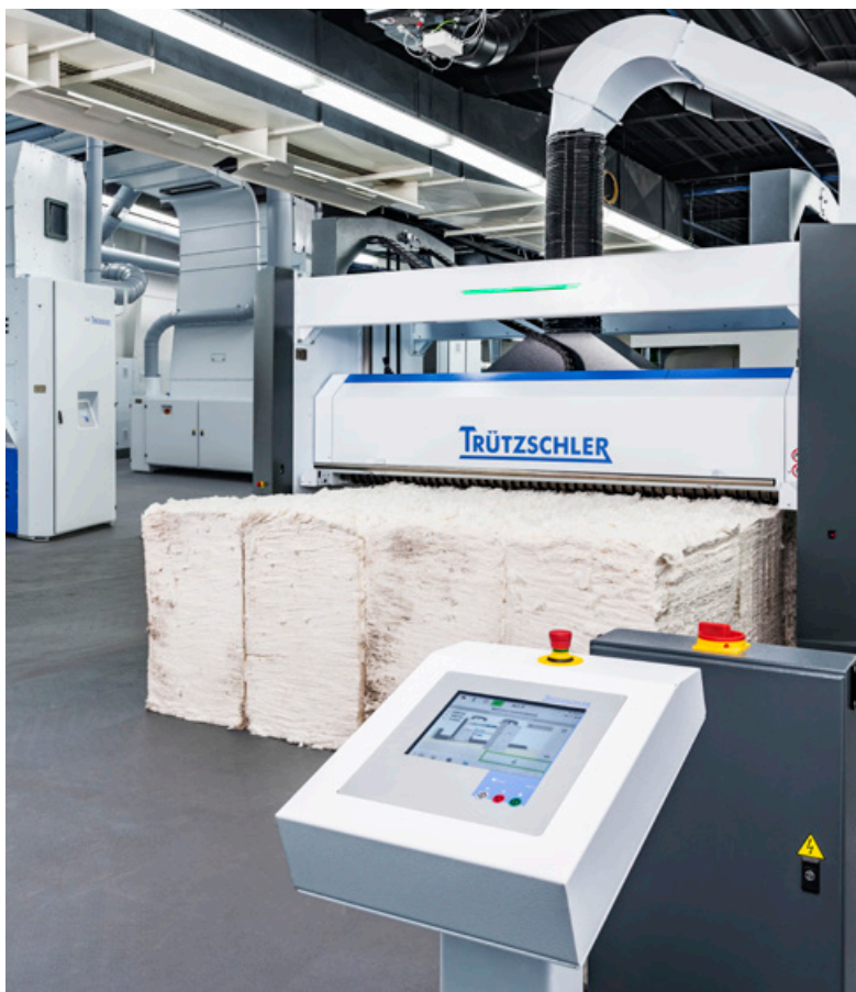
The operating terminal of the Portal Bale Opener BO-P visualises the most important data.
