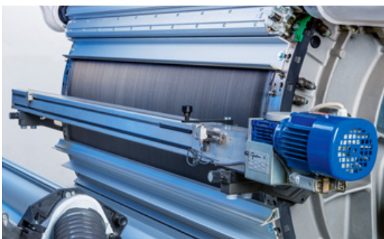
The traversing Grinding Device TC-GD improves carding results for cylinder and doffer.
