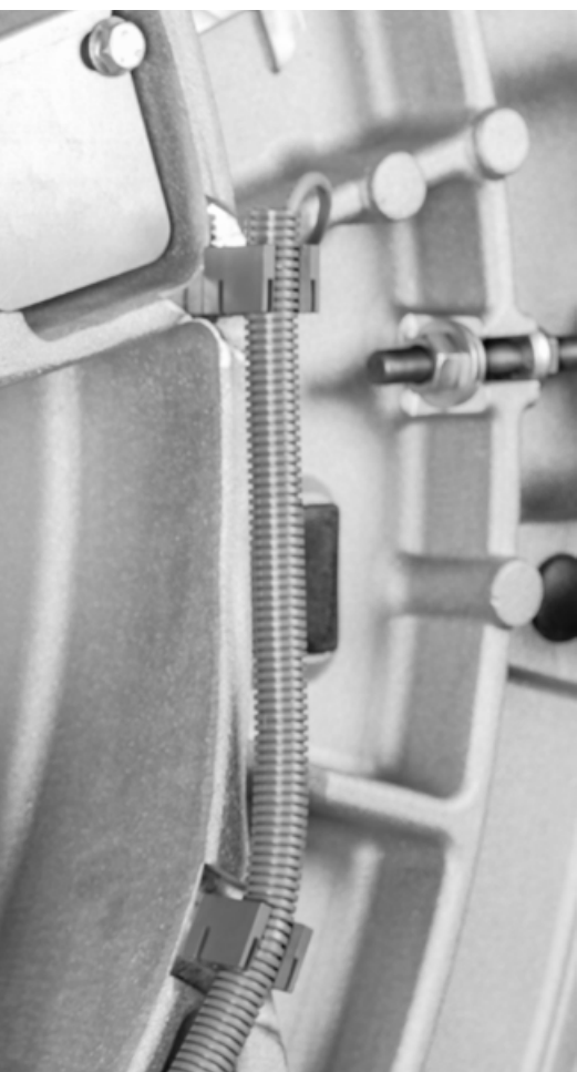
The T-CON 3 spacers can easily be replaced in just a few simple steps and thus allow a reproducible setting of the carding segments.
