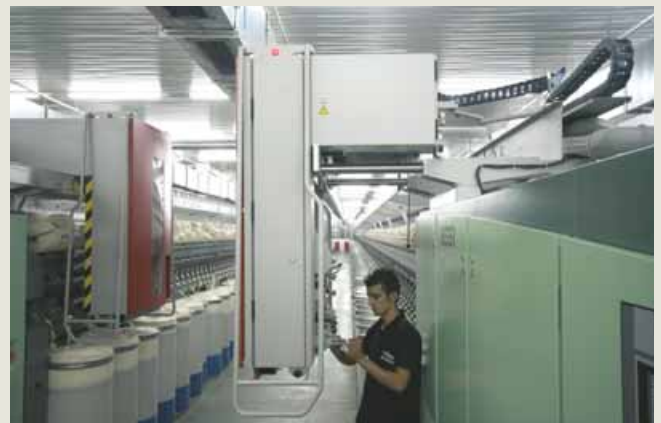
Special service station at the end stock
