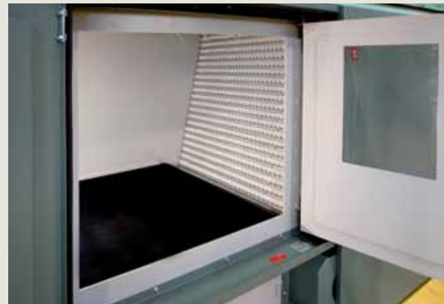
Comfortable access to the conveyor belt and upright lattice
