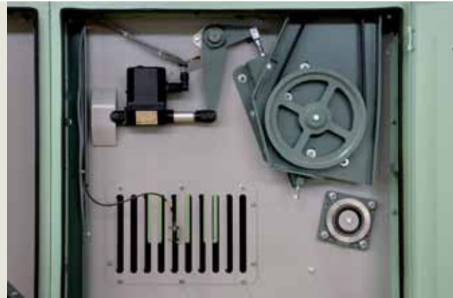
Setting the gap between the blending roller and the upright lattice via an electrocylinder
