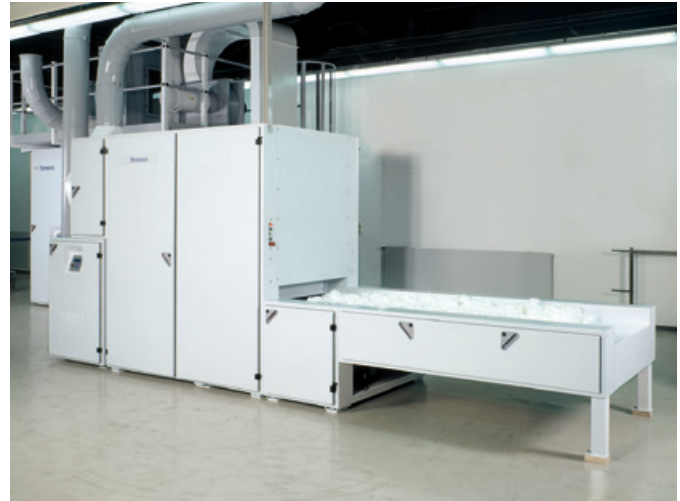
Compact Bale Opener BO-C with Fine Opener TO-C for productions <300 kg/h
