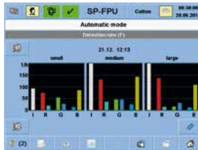
Coloured diagrams show statistics on separation function. Divisions according to size of parts, colour or distribution over machine width facilitate further optimisation.
