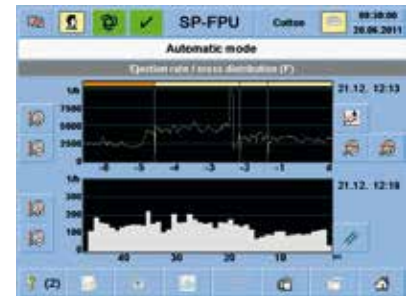
Coloured diagrams show statistics on separation function. Divisions according to size of parts, colour or distribution over machine width facilitate further optimisation.
