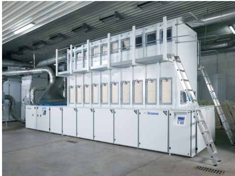
The Integrated Mixer MX-I 10 is directly coupled to a CLEANOMAT Cleaner CL-C 3
