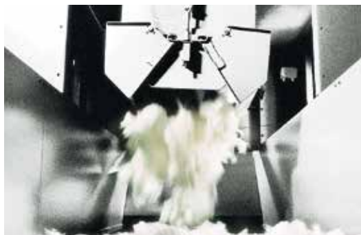
Discharge from a weighing container of the Weigh Pan Bale Opener BO-W
