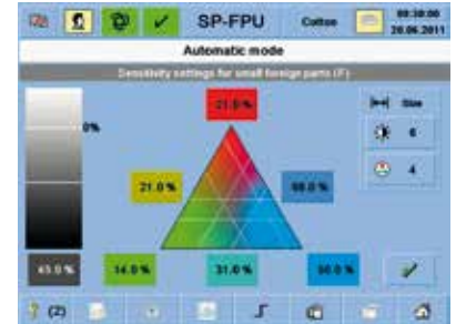
This screen mask is used to activate the basic setting at the touch of a button. Customer-specific optimisation as to part size, contrast and colour are simple to perform.
