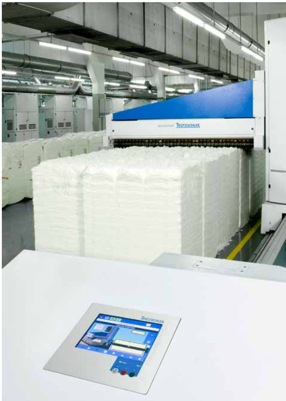
The operating terminal of the Automatic Bale Opener BLENDOMAT BO-A visualises the most important data.
