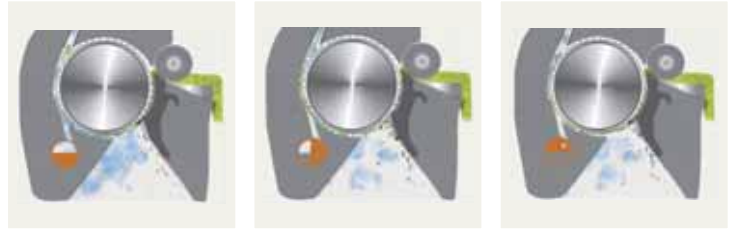
BYpass on the S 60 enables trash extraction to be adjusted for better spinning results
