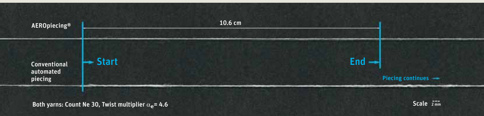
Yarn-like piecings with AEROpiecing® reduce stops in weaving to a minimum
